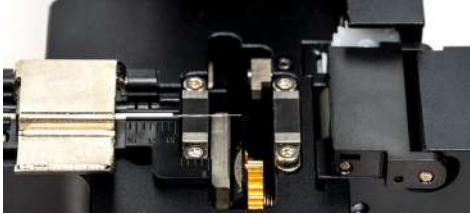
7 - Fix Length & Cleave Fiber (Use FC-600 Fiber Cleaver)
