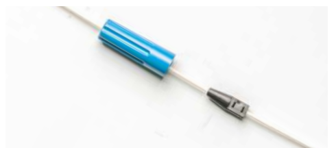
3 - Insert Cable into 0.9 mm Tail Cover
