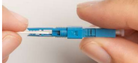
8 - Insert Fiber until it's Slightly Bending
