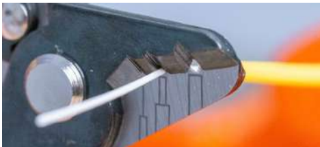
7 - Fix Length & Cleave Fiber (Use FC-600 Fiber Cleaver)
